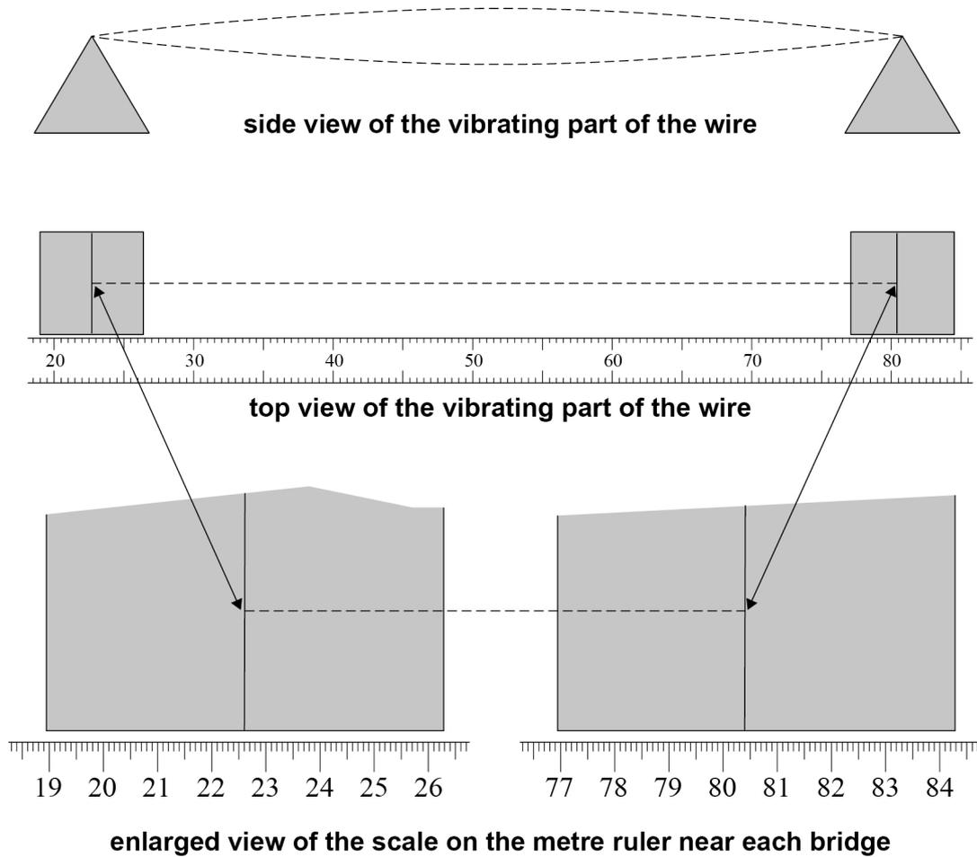
Determine the wavelength  $\lambda$  of the stationary wave shown in **Figure 17**.
