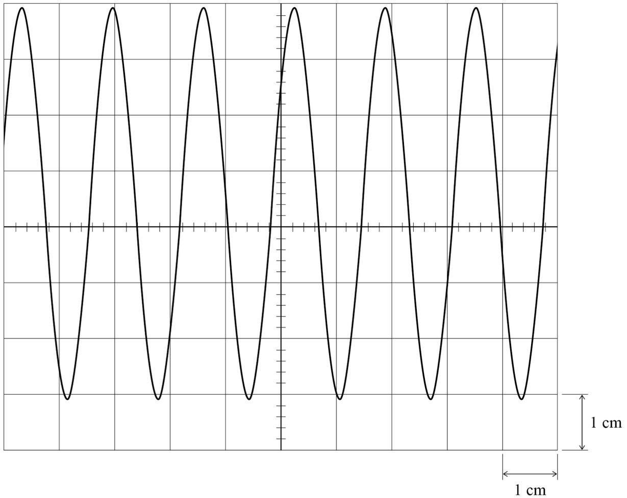
The time-base setting of the oscilloscope is  $10 \text{ ms cm}^{-1}$ .
