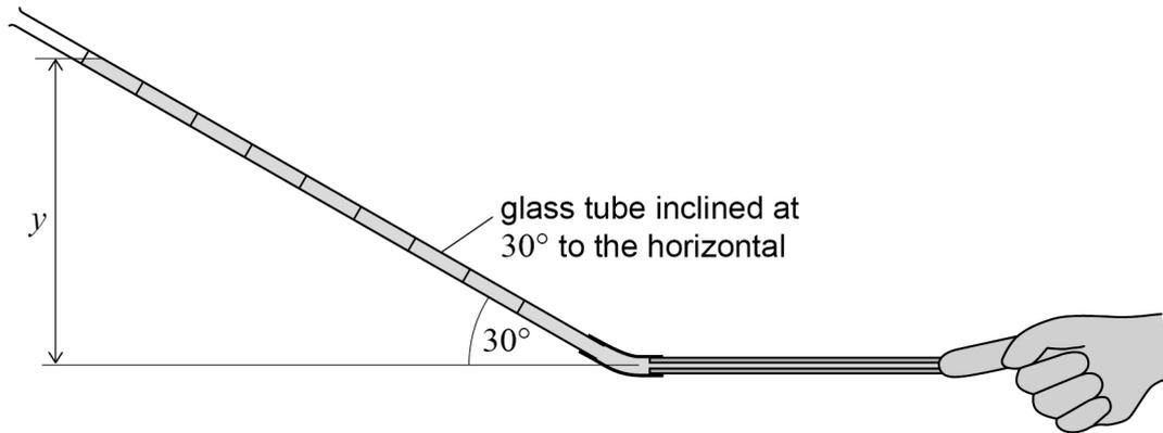
The student measures and records the new values of  $y$ , the mean vertical distance between each of the marks and the centre of **T**. She then carries out the experiment as before, recording new values of  $t$  corresponding to each new value of  $y$ .
