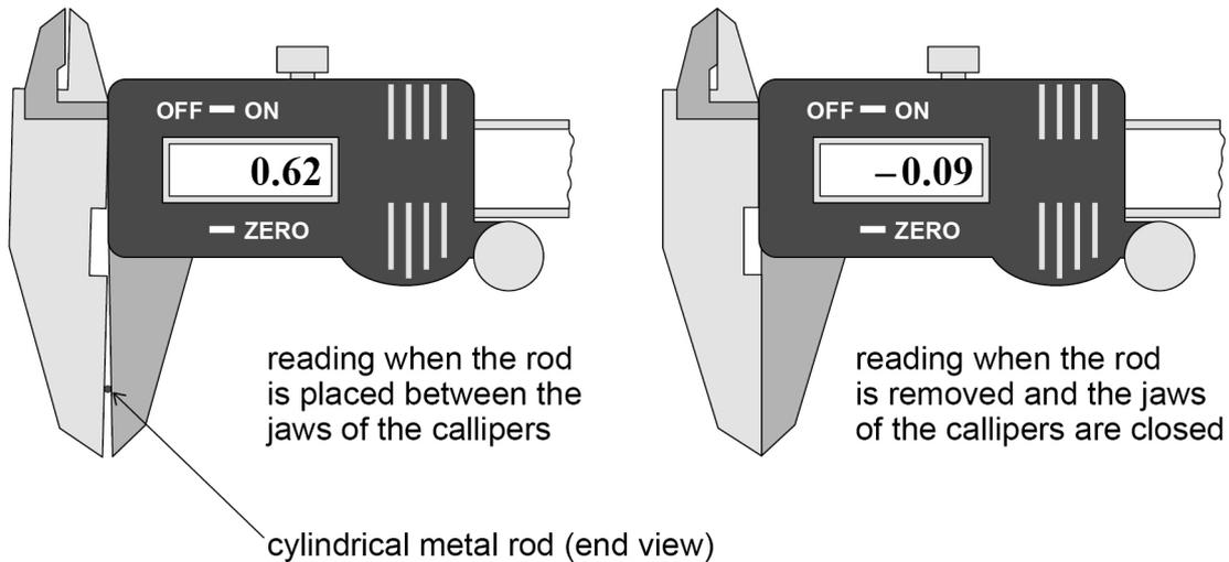
Calculate the diameter  $d$  of the rod.
