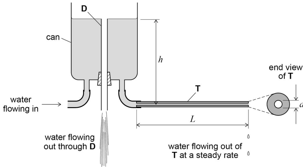
The apparatus ensures that the water level in the can is at a constant height  $h$  above the centre of **T**.
